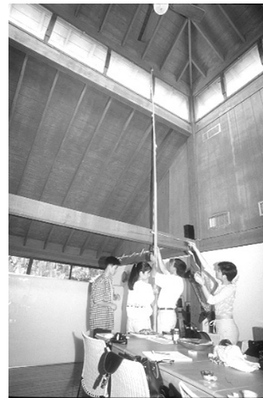
Fig. 3: Team of students negotiate a 20-foot pole to attach a ribbon holding 7 Hobo dataloggers.
