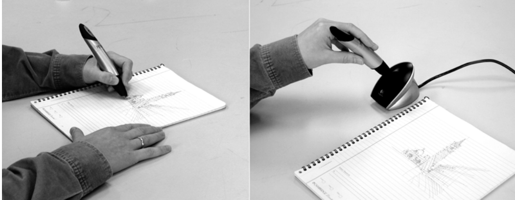
Fig. 1. Drawing with the Logitech Io pen (left) and docking the Io pen to download the information (right).
