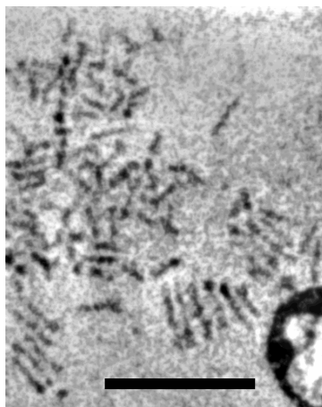
Figure 3-6: CdSe nanorods. TEM magnification was 340 kx and voltage was 120 keV. The scale bar represents 20 nm.
