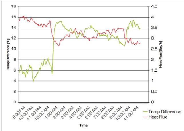
Fig. 5: Graph of heat flux for the moss installed in the window (red) and the temperature difference (green) over time
