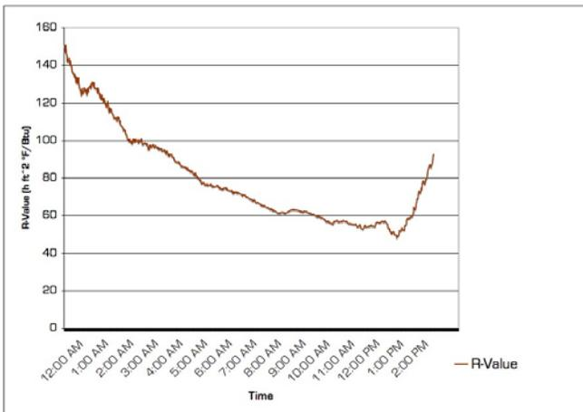
Fig. 7: Graph of calculated R-value of the moss attached to the wall over time.
