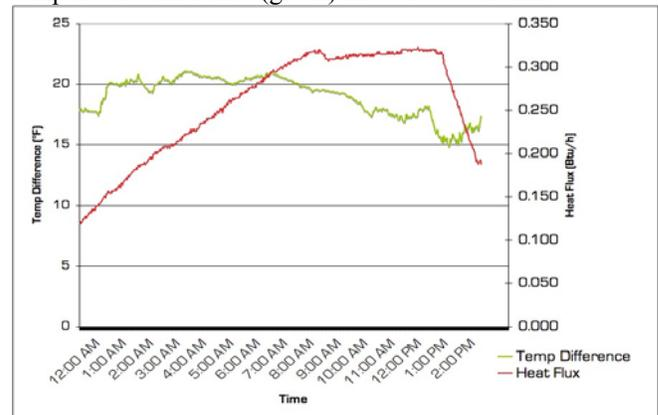
Fig. 4: Graph of heat flux for the moss attached to the wall (red) and temperature difference (green) measured over time.
