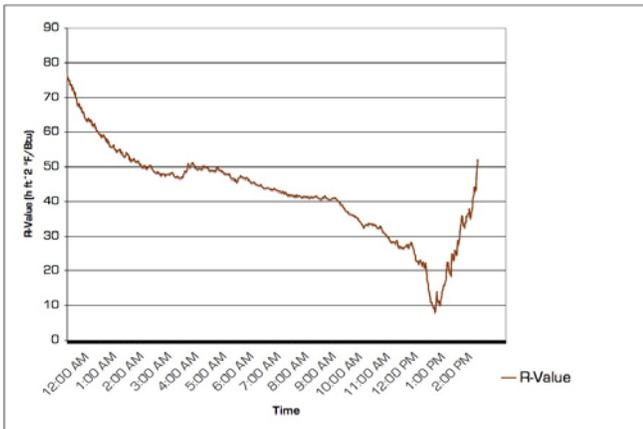
Fig. 6: Graph of calculated R-value of the wall over time.
