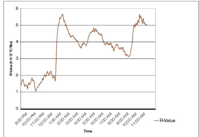
Fig. 8: Graph of calculated R-value of the moss installed in the window over time.
