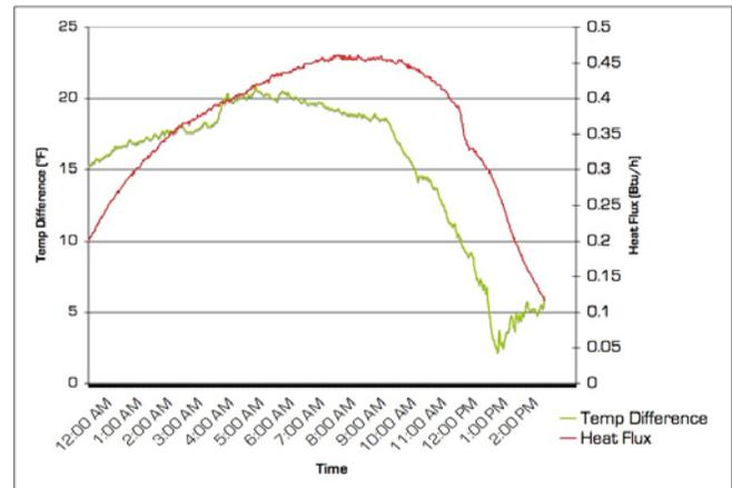
Fig. 3: Graph of heat flux of just the wall (red) and temperature difference (green) measured over time
