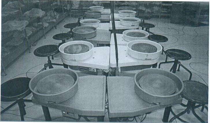
Shimpo VL Whisper potter's wheel (we have 7 of these) Type of power: Electric VOLTAGE: 115V AMPS: 9A WATTS: 400W Hz:60
