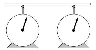
**Observation:** First, place the center of the mass at the 20 cm mark so that it is directly above one scale. Record the support force reading of each scale in the appropriate box in the table below. Continue to fill in the table by moving the mass to different locations on the board. Be careful not to move the board as you are conducting this experiment.
