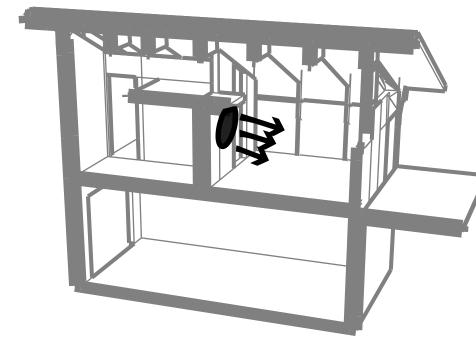
AFTER COLLECTING DATA UNDER NORMAL HEATING CONDITIONS. WE BEGAN TO INTRODUCE MEASURABLE AMOUNTS OF CIRCULATION WITHIN THE APARTMENT. WE PLACED A SMALL HOUSE FAN IN THE SPACE AND RAN IT ON A "LOW" SETTING FOR A TWELVE HOUR PERIOD.
