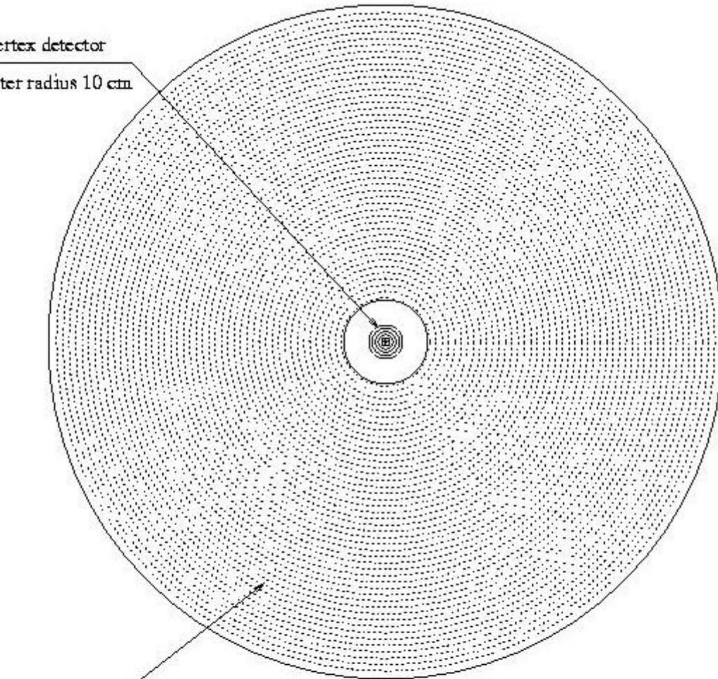
Drift chambers tracker system - 144 layers, outer radius 200 cm.
