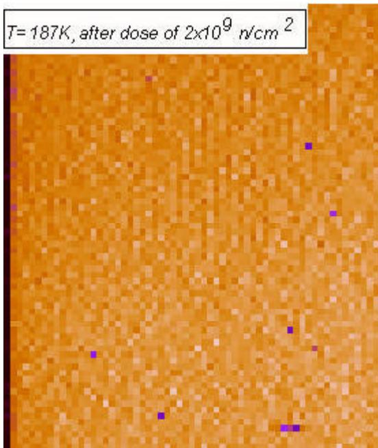
Image of damaged sites after flushing
