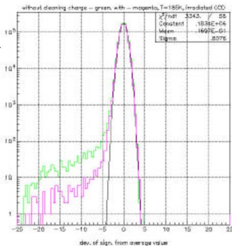
Basic concept demonstrated; future work should involve charge injection to keep traps filled.
