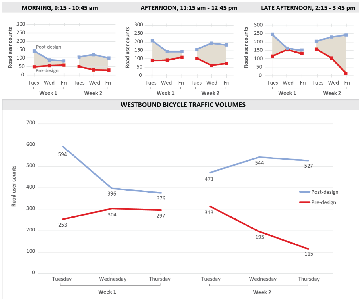
FIGURE 4 Changes in volume of westbound bicycle traffic per time segment and per day.
