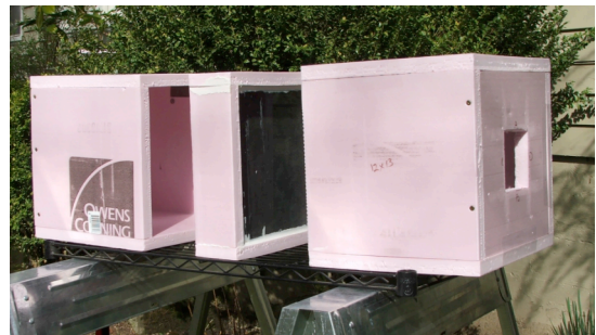
Fig. 1 The constructed simplified “trombe wall” used during testing.
