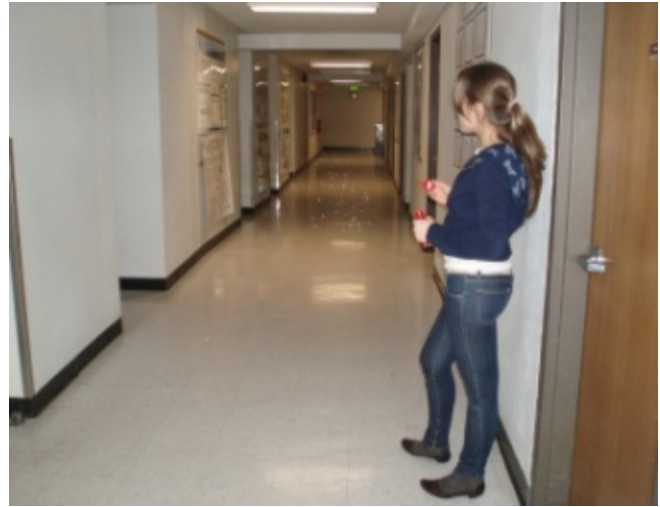
Fig. 1. Testing for wind direction using bubbles.
