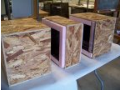
image 1: Completed System With Six Inch Wall.
