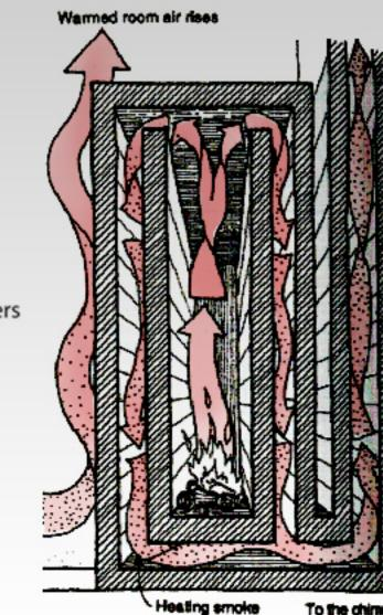
Heating smoke sinks as it cools Modified from Stein, et al. 2005 p. 334
