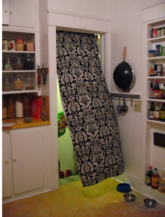
Figure 6: Blower door fan pulling curtain into the main kitchen/living area.
