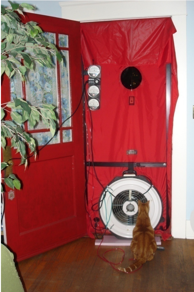
Figure 5: Blower door & Nitro.
