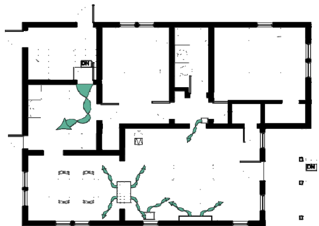
Figure 9: Locations of Major Infiltration Sources
