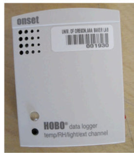
Hobo Data Loggers - 4 total (2 on each side of window)
