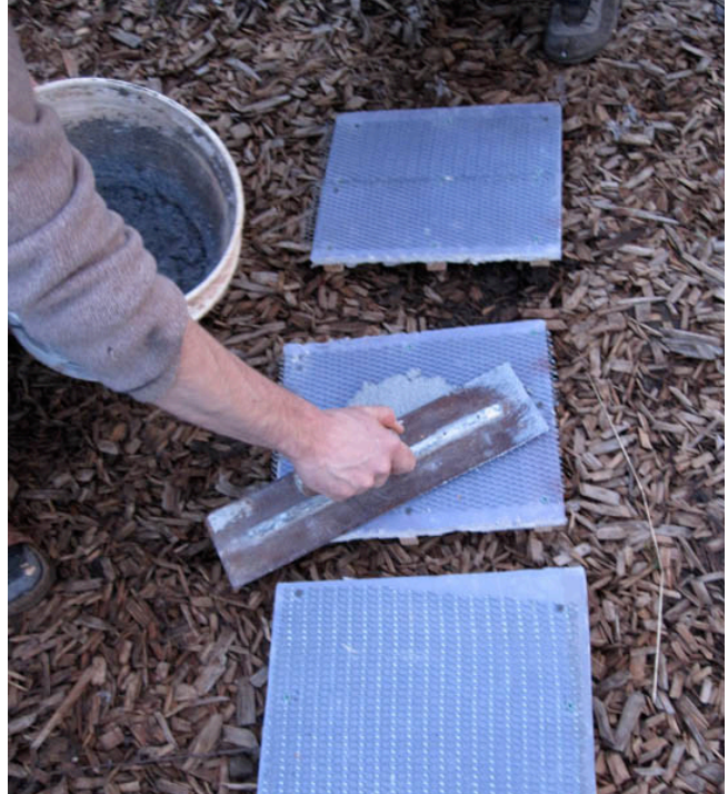
Fig. 5: Troweling plaster on test square
