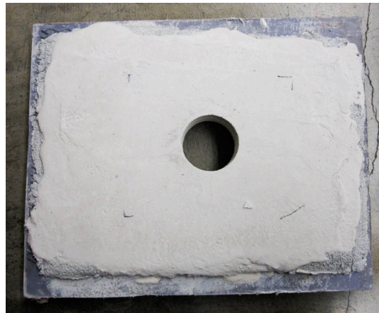
Fig. 9: Test sample post drilling
