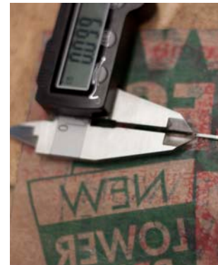
Figure 4b. Tear measurement using electronic calipers
