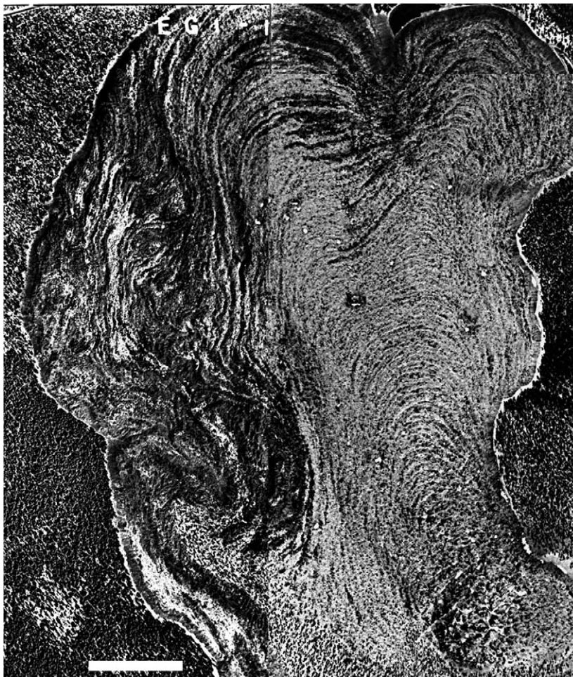
Fig. 3. Aerial photograph mosaic of the Big Obsidian Flow showing arcuate flow ridges concave toward the vent. Dark lava is CVP while light gray lava is FVP. Scale bar represents approximately 300 m.
