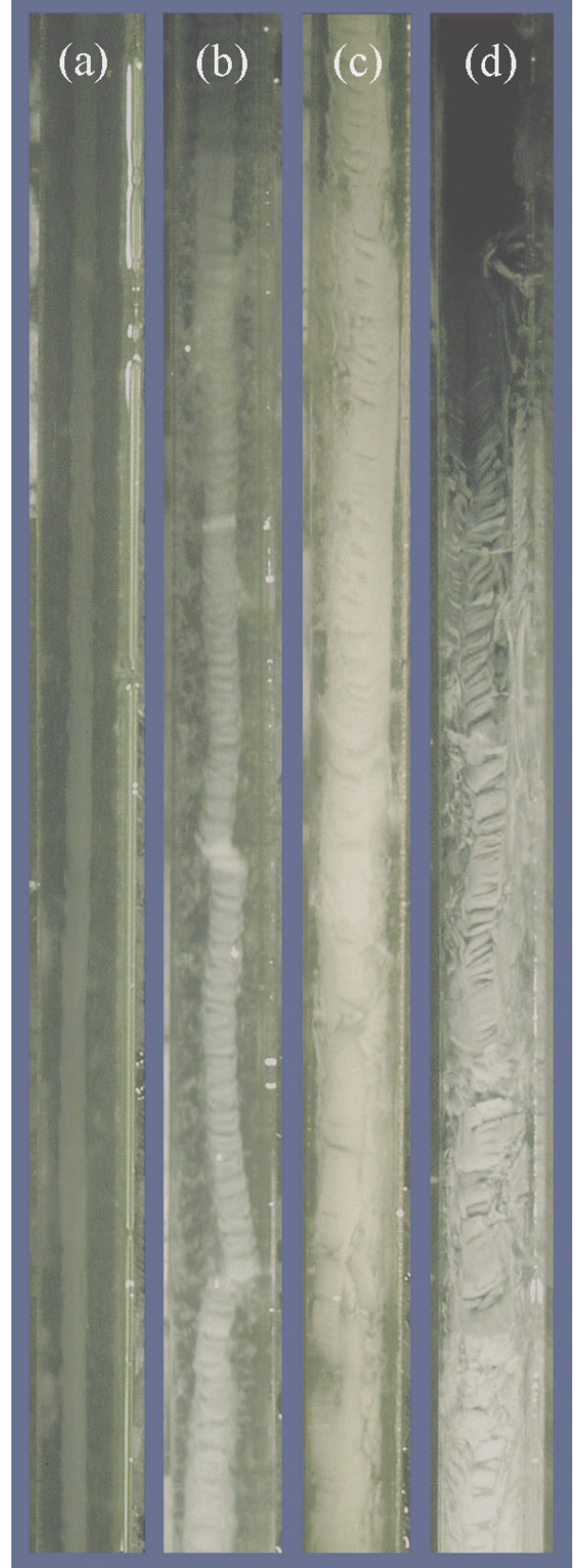
Figure 2. Photographs showing the extent of solid in the 44 mm wide channel under conditions ranging from: (a) \psi r = 3.1, r = 0.82 ; (b) \psi r = 2.2, r = 0.57 ; (c) \psi r = 0.92, r = 0.34 ; (d) \psi r = 0.43, r = 0.33 . Solid wax is white, liquid PEG is transparent and the base of the tank is painted black. Flow is from top to bottom. The photographs correspond to
