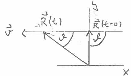
$\rightarrow$  For fixed distance  $R$  from the charge,  $\vec{E}$  is minimal for  $\theta = 0, \pi$ , i.e., in the direction of the motion. This minimal value is
