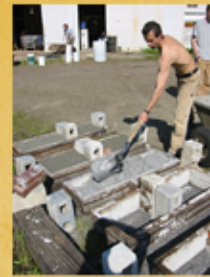
2. Care must be taken at this stage not to compress the mix too much. It diminishes air pockets thereby reducing insulative performance.
