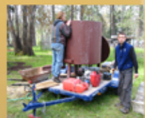
Yeti peers into a state-of-the-art, custom 300 gal. papercrete mixer. Peter is very impressed.
