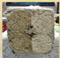
A Green Beam consisting of four spindly bales of straw bound together and encapsulated with papercrete. (Load resisting characteristics were questionable)
