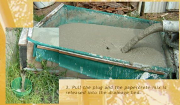
A rain gutter catches the excess water and routes it to a bucket set in a hole. This water is reused for subsequent batches. It also runs fairly clear, leaving desired solids behind.
