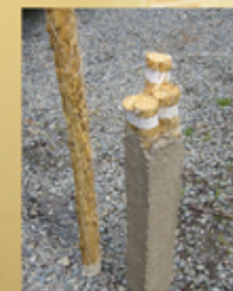
Ashland team's formwork with integrated mesh for drainage and ventilation.
