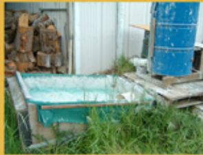
2. The paper slurry and additives are poured into this 55 gal. drum mixer and blended. To the left of the drum is the drainage bed, where excess water is removed and sand added to the mix by hand.
