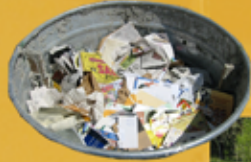
2. Jodi adds water to the paper in the tow mixer, a 200 gal. drum with a lawn mower blade mounted in the bottom.
