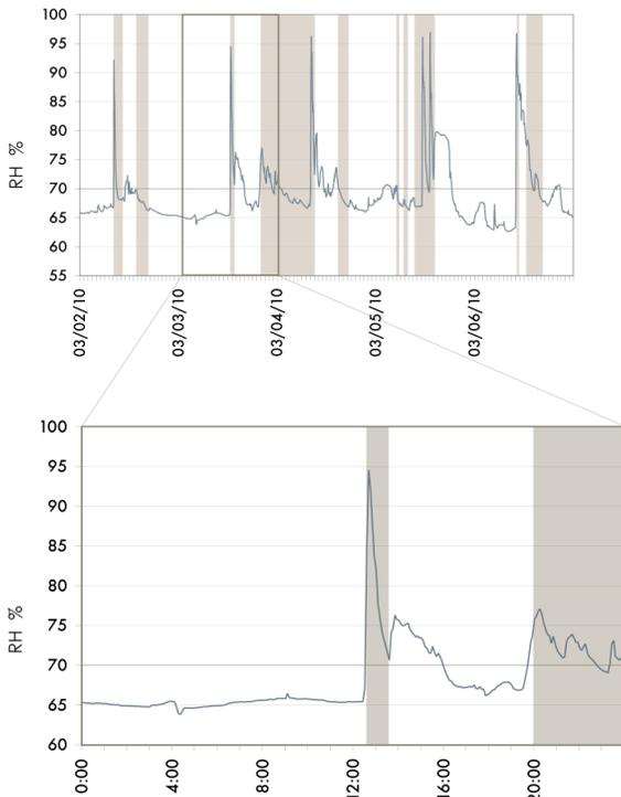
Fig. 11: Weekly and daily conditions with the dehumidistat-controlled fan.
