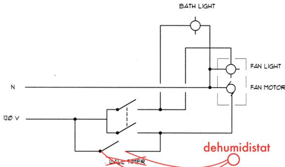
Fig 7: Wiring diagram with dehumidistat
