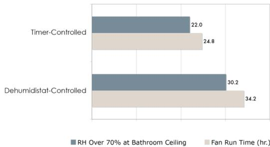
Fig. 8: Total fan run time and time spent over 70% RH
