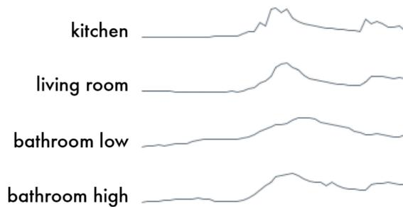
Figure 12: Evening baking's effect on apartment RH
