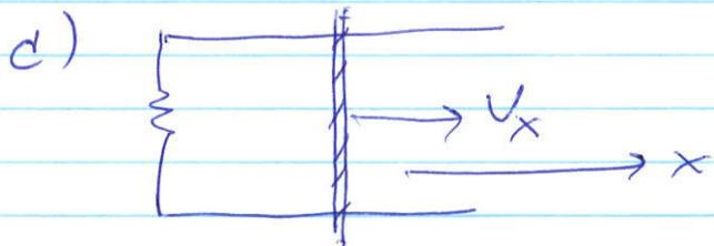
$$m_{bar} \ddot{v}_x = -Ib_0 l = -\frac{v_0 B^2 l^2}{R}$$
