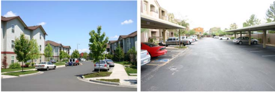
Figure 4. Development organized around a defined, multimodal street network that includes on-street parking, buffers from moving cars, and buildings facing the street (left), compared to a more typical development organized along wide, auto-dominated parking lanes (right).
