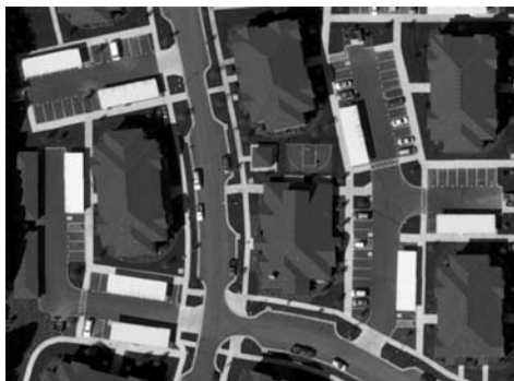
Figure 5. Parking pods (along the right and left sides of the image) provide additional parking off the street network. Pods are limited in size and do not allow through traffic. Also notice the robust street network that serves the buildings, street, and parking areas in this development.
