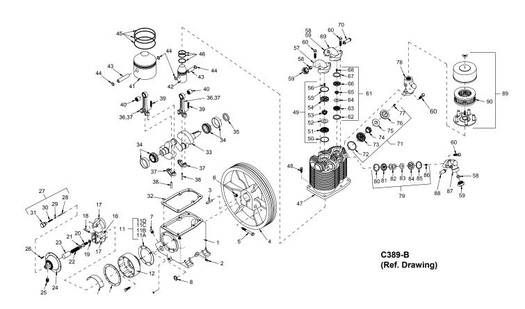
Repair Parts List Compressor Models R10D & R15B
