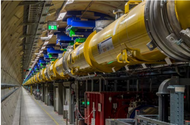
FIG. 9: View of installed cryomodules in the tunnel of the E-XFEL [58].
