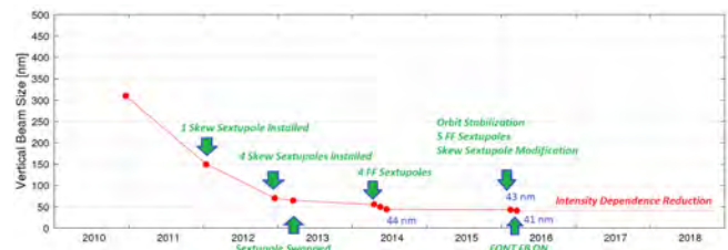
FIG. 15: Beamsizes achieved at the Accelerator Test Facility 2 (ATF2) as a function of time [92]. The latest result (41 nm [88]) is within 10% of the goal beam size of 37 nm.
