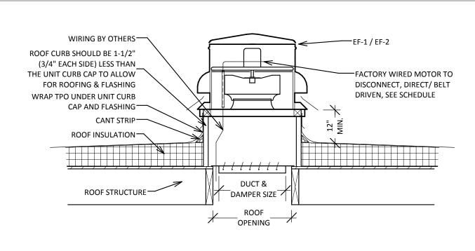
SPUN ALUMINUM EXHAUST FANS SHALL BE CENTRIFUGAL DIRECT BELT DRIVE TYPE. THE FAN WHEEL SHALL BE CENTRIFUGAL BACKWARD INCLINED, CONSTRUCTED OF ALUMINUM AND SHALL INCLUDE A WHEEL CONE CAREFULLY MATCHED TO THE INLET CONE FOR PRECISE RUNNING TOLERANCES. WHEELS SHALL BE STATICALLY AND DYNAMICALLY BALANCED. THE FAN HOUSING SHALL BE CONSTRUCTED OF HEAVY GAUGE ALUMINUM WITH A RIGID INTERNAL SUPPORT STRUCTURE.
