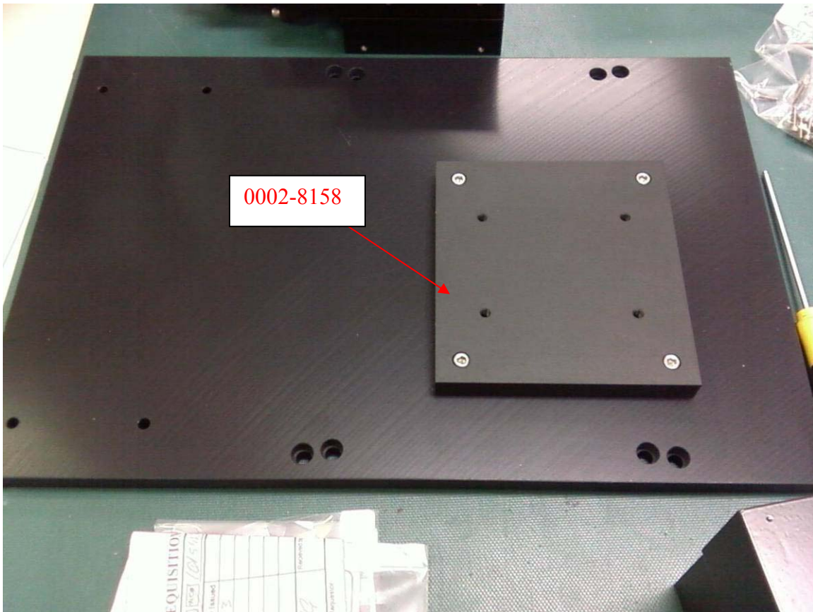
Attach plate (I) to plate (H) by using four 10-32 X 1/2 (PN 2825-6956) SHCS screws.
