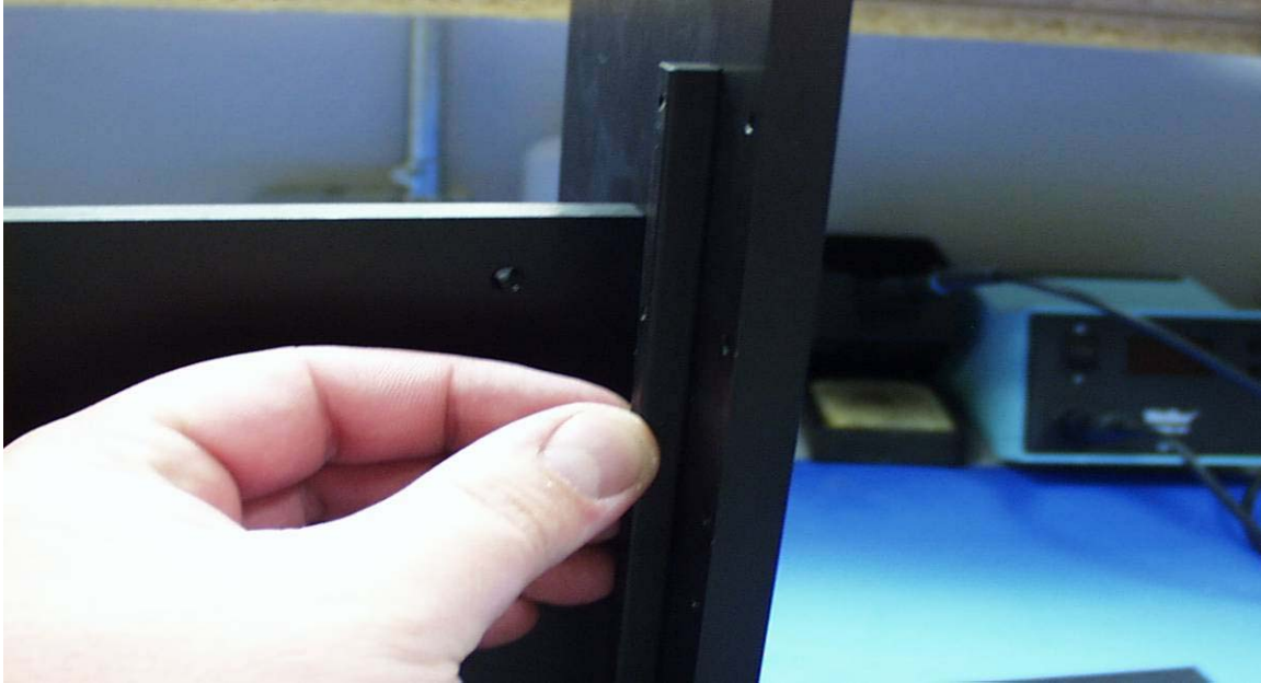
Install (2) Weight Guides (L)–one on each side of C & D–with 4-40 X 1/2 (2825-6736).
