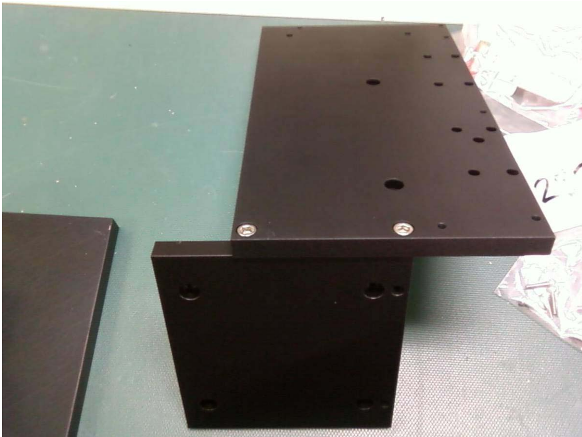
Attach Plates with 2825-6957 SCR,SKT HD,CAP,10-32X5/8,SS On both sides
