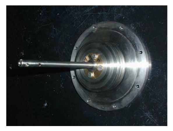
Reassemble with the new bellows by following the procedures in reverse.
