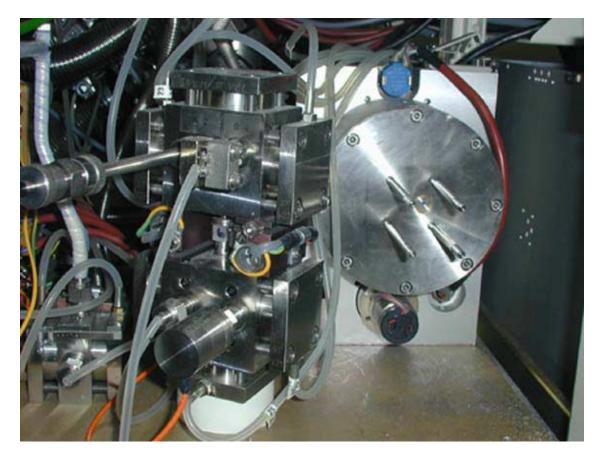
\*\*\*Please note the small gold gasket in the recessed port in this picture. A new gasket will be required during reassembly. \*\*\*
