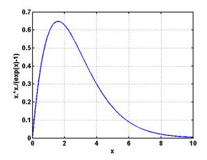
Graphically (a good, quick way to do evaluate the integral) we see that the area under the curve covers about 13 boxes of area 0.2, so the integral  $\approx 2.6$ .
