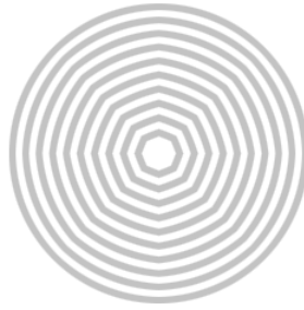
Figure 1.6. Wavefronts for a spherical wave are concentric spheres centered on the source.
