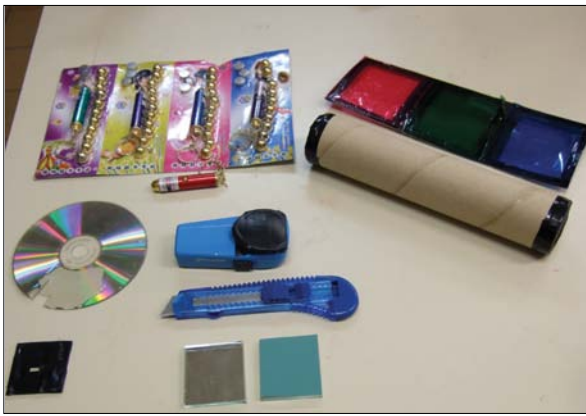
Fig. 13. Low-cost equipment for ALOP: lasers, diffraction gratings from discarded CDs, slits scratched into coated mirrors, cellophane color filters, and spectrometer from a diffraction slide.
