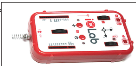
Fig. 1. The IOLab, an inexpensive data acquisition device in a cart that can roll on its three wheels.
