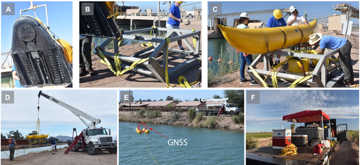
Figure 2. Photos of compressed high-intensity radar pulse (CHIRP) instrument deployment. (A) Transducers on CHIRP bottom. (B) CHIRP frame. (C) Buoyant pontoons to float frame. (D) Deployment of CHIRP from northern canal bed. (E) Towing CHIRP from the southern bank with a towline; umbilical and second towline (right) toward the northern bank and topside. Global navigation satellite system (GNSS) receiver on frame mount (red circle and arrow). (F) Topside system setup.
