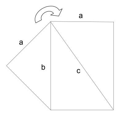
Magic mirror layout. a determines b, which determines c.
