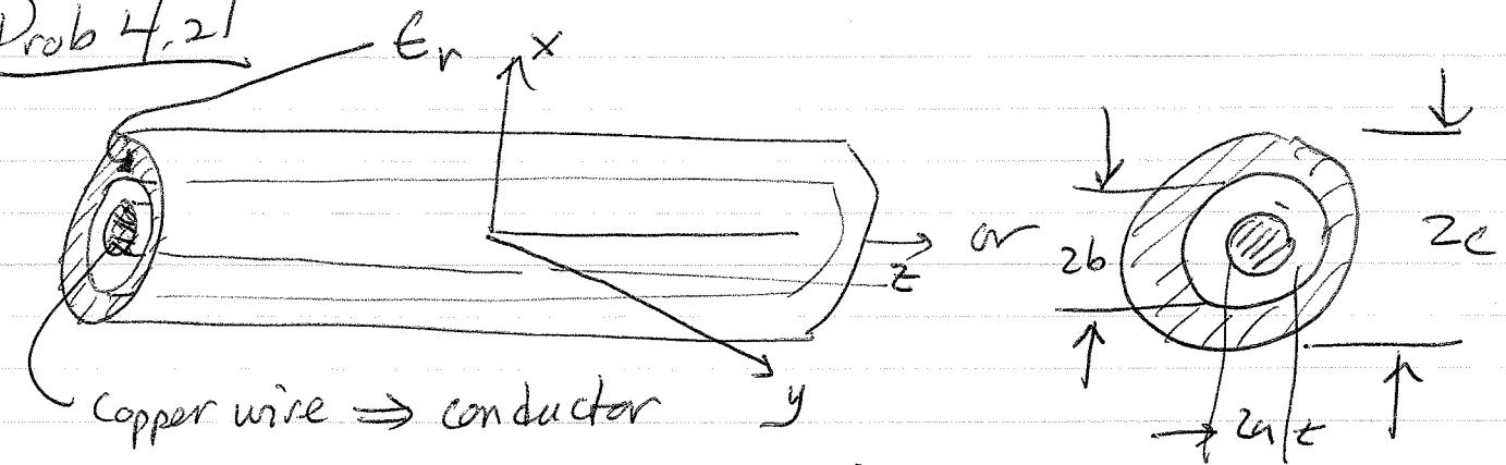
Find the capacitance of this coaxial cable.
