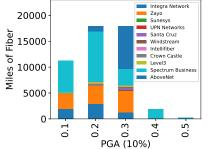
**Fig. 7.** Miles of fiber affected for expected PGA with 2% probability.
