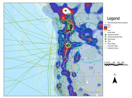
Fig. 2. Internet infrastructure overlap with mapped faults (yellow dotted lines) in PNW.
